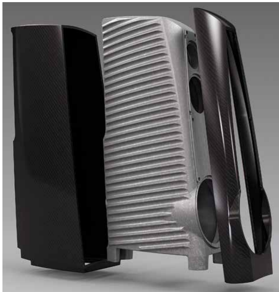
ABOVE: The three major components of the Orion's enclosure are seen here – an inner cast alloy shell, with ribbing and internal bracing, sandwiched between an outer carbon-fibre/polyester carapace and baffle plate [see p43]
